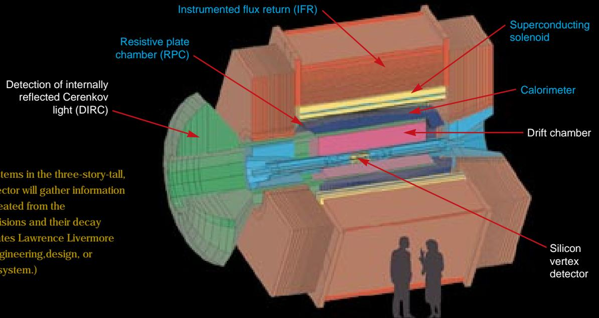
**Figure 2.** The subsystems in the three-story-tall, 1,000-ton BaBar Detector will gather information about the particles created from the electron-positron collisions and their decay products. (Blue indicates Lawrence Livermore involvement in the engineering, design, or fabrication of the subsystem.)
