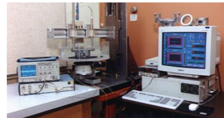
Figure 2. Prototype ultrasonic scanning system (with sample pistons atop the monitor) that will be used for detecting very small casting defects.
