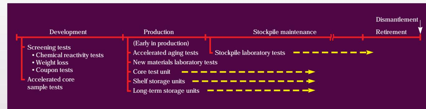
Figure 1. Phases of evaluation in stockpile surveillance.
