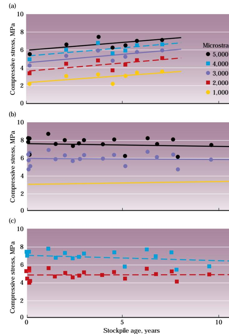
Figure 4. (a) The compressive stress tests for the LX-17 high explosive recovered from the W87 new materials laboratory test (NMLT) units and stockpile laboratory test (SLT) units. The data show a stiffening of the LX-17 at all strain levels, which may be consistent with a gradual increase in the crystallinity of the Kel-F-800 binder. For reasons not clear at this time, this trend is not supported by the observations from the B83 (b) NMLT units and (c) SLT units.
