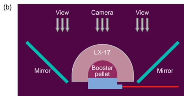
**Figure 5.** (a) A "snowball" test assembly (bottom) is aligned with samples of snowball test data (top) as recorded by the streak camera. (b) The schematic shows the mirrors that reflect the left and right sets of snowball data.
