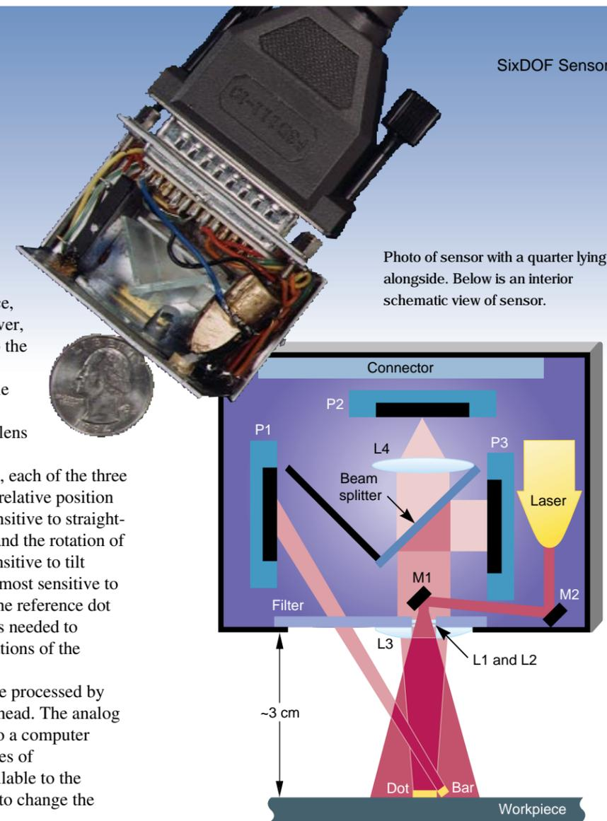
Photo of sensor with a quarter lying alongside. Below is an interior schematic view of sensor.
