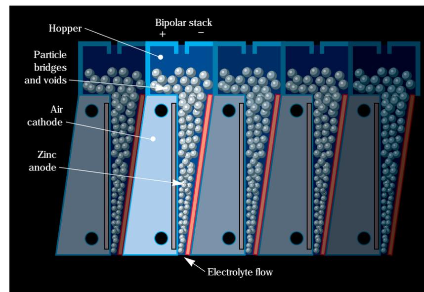
**Figure 3.** Zinc pellets are gravity fed from hoppers to cells.
