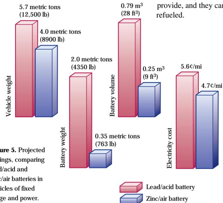
**Figure 5.** Projected savings, comparing lead/acid and zinc/air batteries in vehicles of fixed range and power.
