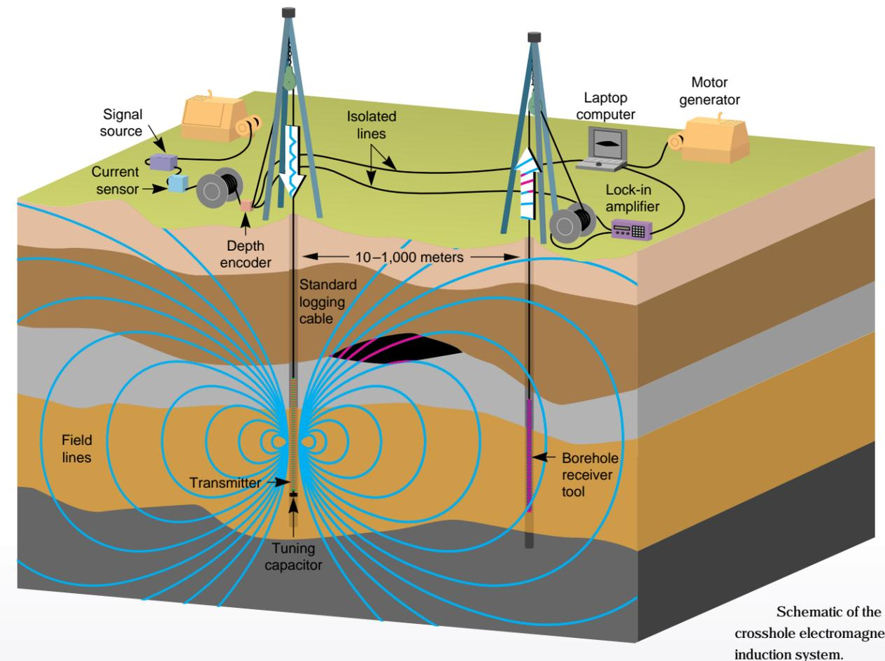
Schematic of the crosshole electromagnetic induction system.
