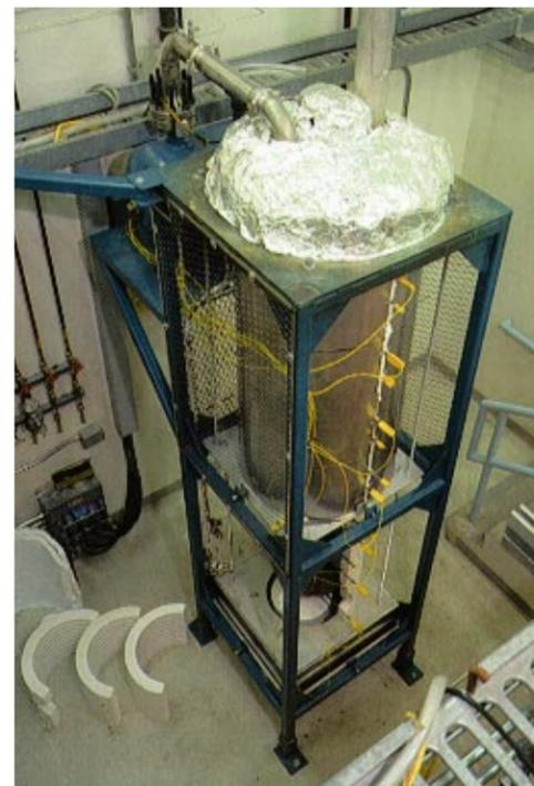
A view of the molten salt crucible and associated piping from above. The slurry of waste and air enters the top of the crucible, and off-gases exit through the larger pipe on the right.
