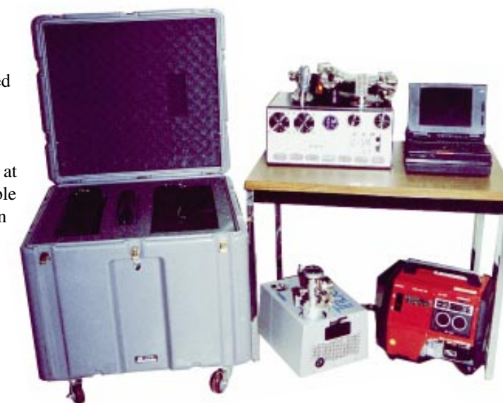
All of the traveling components of LLNL’s miniaturized gas chromatograph/mass spectrometer can fit into a metal travel case. Included are (on table) the GC/MS and laptop computer and (on floor) the pumping unit and generator.
