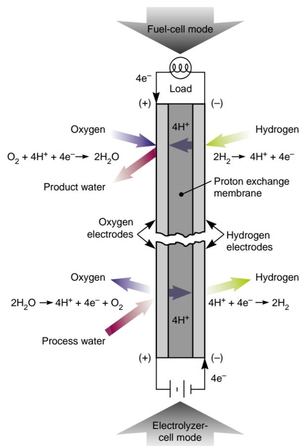
**Figure 1.** The electrochemistry of a unitized regenerative fuel cell. In the fuel-cell mode, a proton-exchange membrane combines oxygen and hydrogen to create electricity and water. When the cell reverses operation to act as an electrolyzer, electricity and water are combined to create oxygen and hydrogen.
