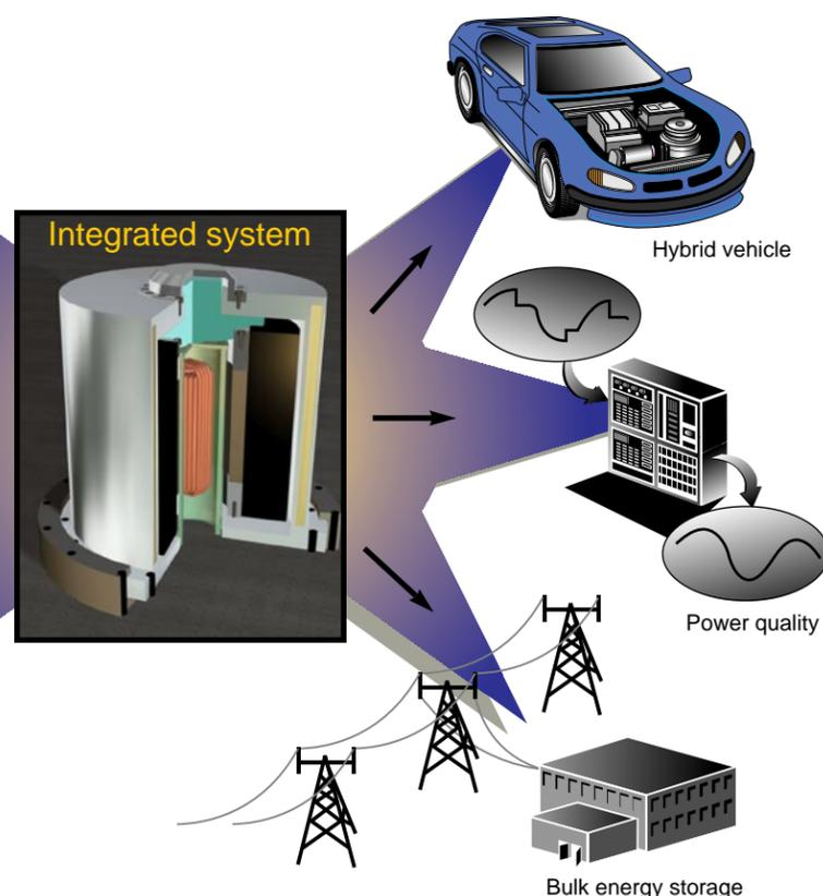
Figure 2. Concept of the flywheel battery system and its applications.
