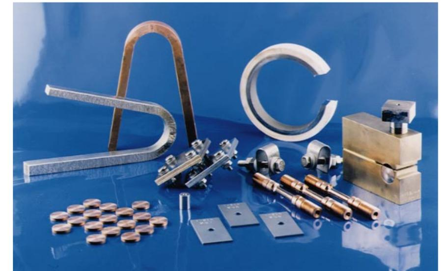
**Figure 6.** Some of the thousands of metal alloy samples we are subjecting to stress, heat, water, and chemicals to determine their long-term performance: penny shapes of copper for electrochemical disks, stainless steel U bends for stress-corrosion tests, a ring of plasma-sprayed carbon steel, and large U bends of pure copper and copper-nickel for aggressive tests of welded samples.
