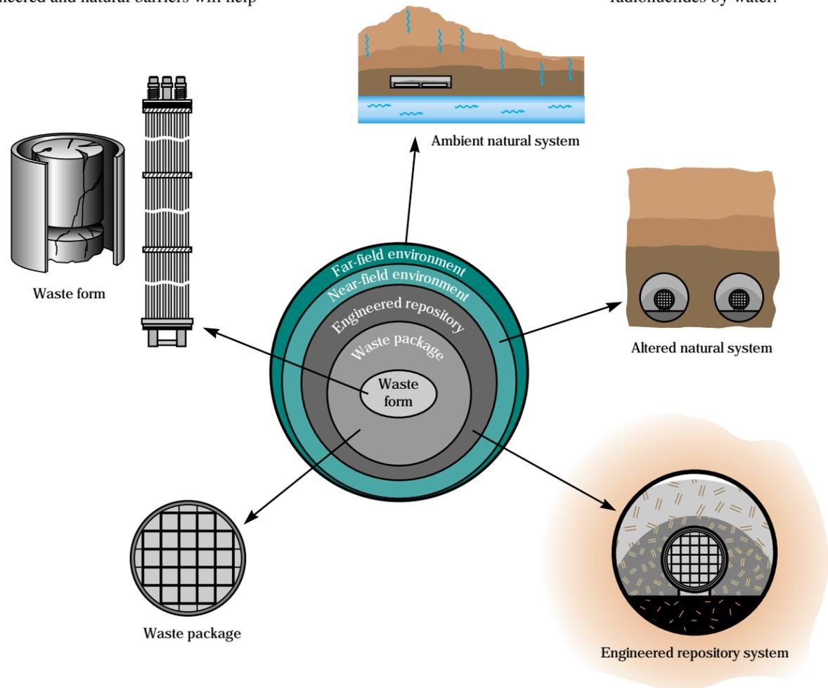
**Figure 2.** The performance of a nuclear waste repository depends on a system of manmade and natural barriers that will delay the release of radionuclides over thousands of years. LLNL's primary responsibilities include selecting materials for the waste package and assessing interactions with the near-field environment extending several hundred meters into the rock.
