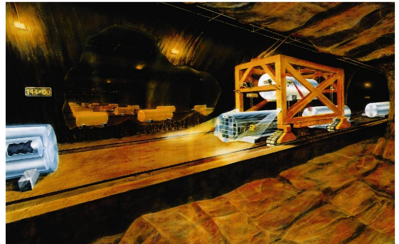
**Figure 4.** Waste packages will be placed on rails in horizontal tunnels, called drifts, about 300 meters underground. The tunnels would remain open for 100 years to permit monitoring and to allow for retrieval if a problem is discovered or if some use is found for the spent fuel. After that period, the tunnels would be filled and sealed.
