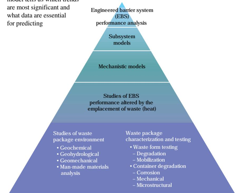
**Figure 8.** Summary of LLNL's role in repository research. Starting with the waste package (bottom right) and our near-field studies (bottom left), we are developing models for evaluating the total performance (top) of an engineered barrier system.
