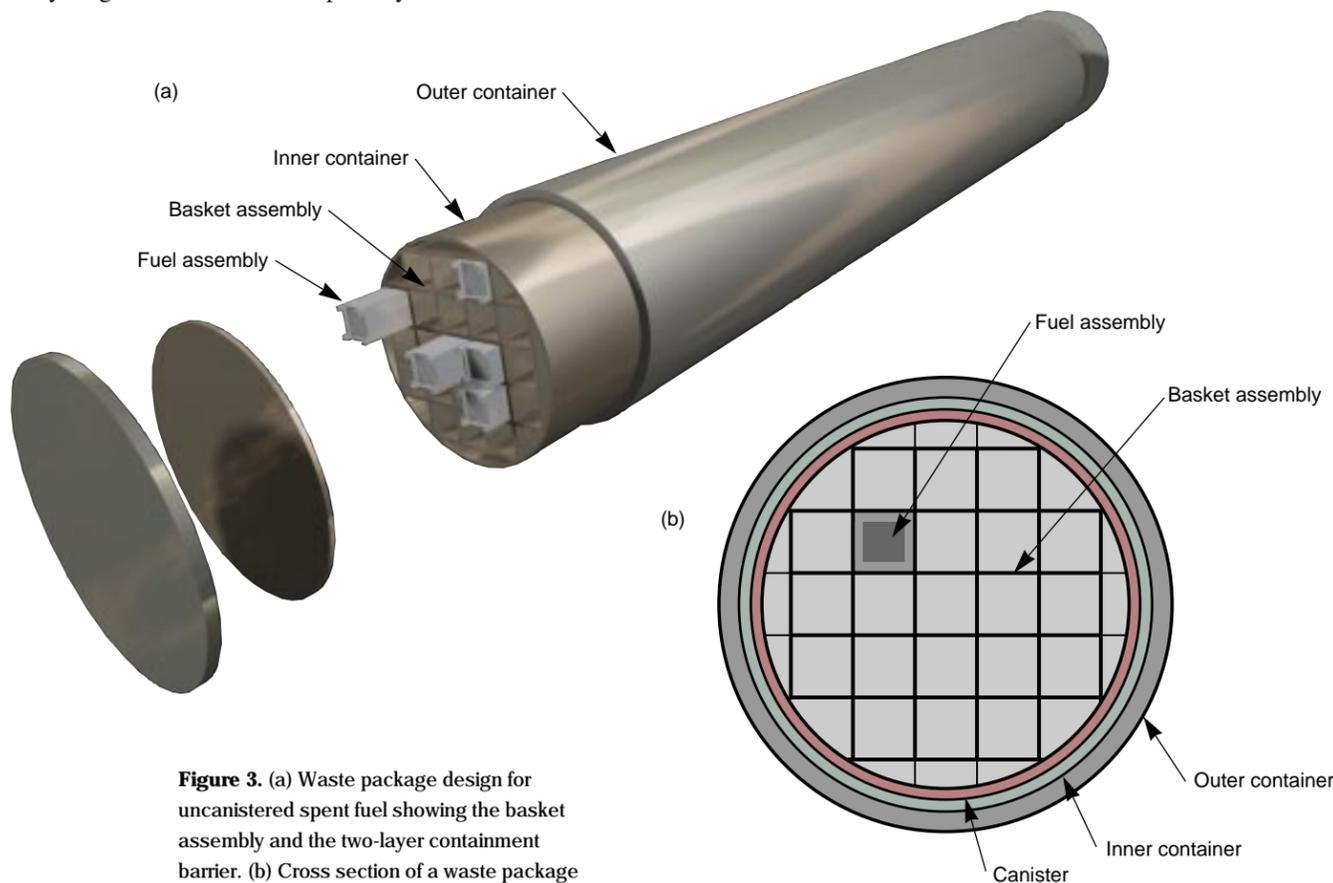
**Figure 3.** (a) Waste package design for uncanistered spent fuel showing the basket assembly and the two-layer containment barrier. (b) Cross section of a waste package containing a multipurpose canister used for transportation, storage, and disposal.
