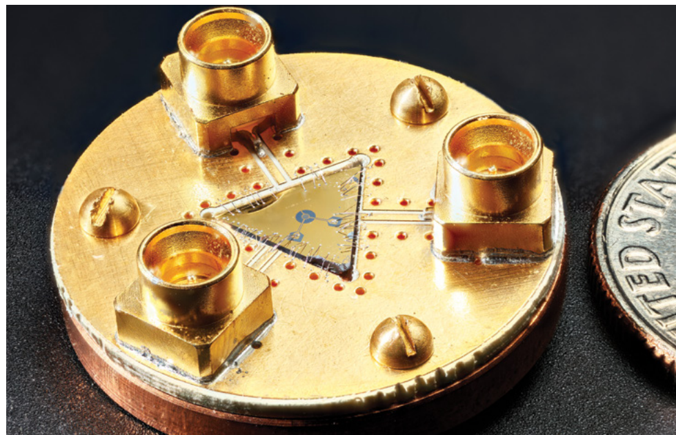
Noise handling is paramount in quantum devices. This 3-port, on-chip microwave circulator is under development at Livermore. Designed from topological materials, control signals enter one port (large cylinders), and the noise produced from operating a connected device, such as a qubit, is diverted out an adjacent channel via the other ports. The circulator (small dark circle) is 1,000 times smaller than traditional bulk circulators. (Dime included for scale.)
