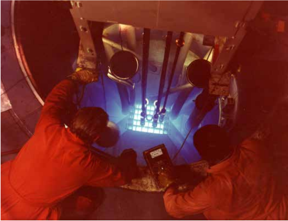
Livermore scientists in the 1970s insert experimental test samples into the LPTTR's core.
