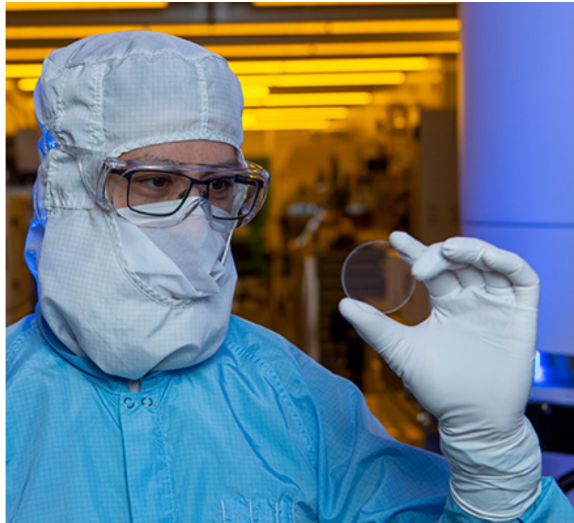
Staff scientist Nathan Ray holds a fused silica optic whose engineered surface features instill antireflective properties. The optic's all-glass metasurface is composed of millions of nanoscopic structures.
