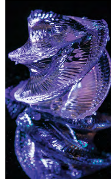
The tailored glass by direct ink writing technique preserves fine features while exercising free-form flexibility, as in this 3D-printed helical glass structure.
