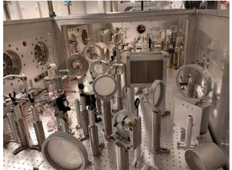
The Berkeley Lab Laser Accelerator (BELLA) Center supported work to perform x-ray tomography of high-Z components. Optics in the foreground channel electron and laser beams that are fired toward a sample staged at the far side of the setup.
