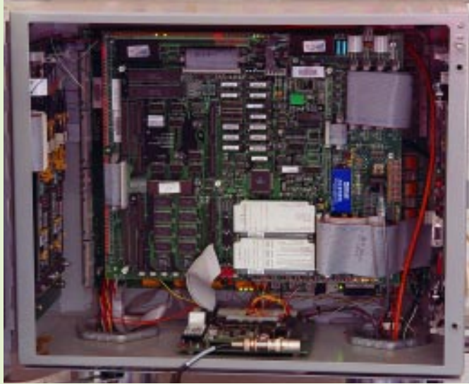
Figure 2. Argus field processors are microprocessor-based devices that verify badge information transmitted from remote access panels against locally stored encrypted access authorization databases.
