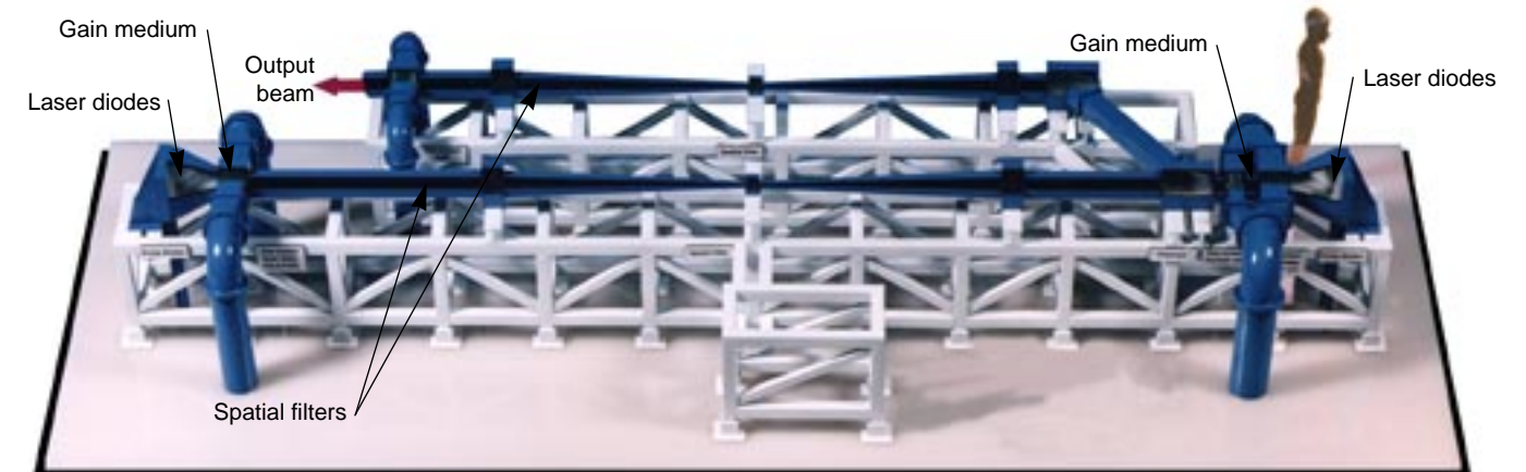
Figure 2. Model of a 1-kilojoule future "beamlet," based on diode-pumped solid-state laser technology, gas cooling of the laser slabs, and ytterbium-doped strontium-fluorapatite gain medium.
