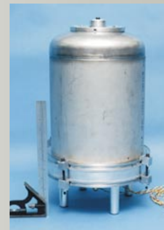
Figure 1. Prototype of the LLNL electromechanical battery, which is based on the flywheel concept of energy storage. Left to right: high-speed rotor, rotor in motion, and enclosed battery (20 cm in diameter by 30 cm high).
