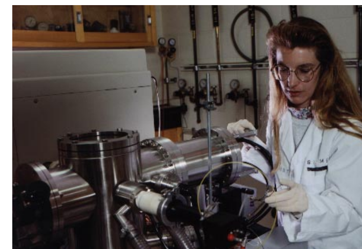
Figure 6. Kathleen Dewhirst combines methods, such as gas chromatography and mass spectrometry or liquid chromatography and mass spectrometry, to characterize the food mutagens in cooked meat. Mass spectrometry allows us to determine the molecular weight of a mutagen.
