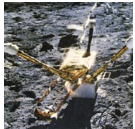
(E&TR November 1976 ) The lunar surface magnetometer deployed at the Apollo 16 landing site. The boot prints indicate scale. The golden ribbon is a power and signal cable. Together with an orbiting magnetometer aboard Explorer 35, this and other instruments provided a continuous record of changes in the magnetic field on the Moon over many months. (NASA Apollo photo.)
