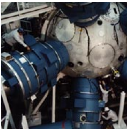
( E&TR February 1985) The Nova target chamber, a massive aluminum sphere 4.6 m in diameter with walls almost 13 cm thick. The large flanges carry the frequency-conversion arrays and the final focusing lenses with their positioning mechanisms.
