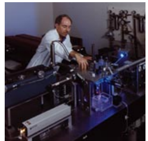
(E&TR April-May 1992) A flow sorter designed and built at LLNL for high-speed sorting of human chromosomes in our Human Genome Center. This sorter features three lasers, state-of-the-art optics, and the latest computer technology, which together produce a versatile and powerful research tool for measuring the level of genetic injury in human cells.
