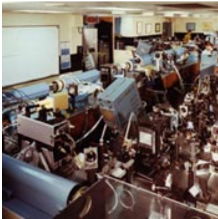
(E&TR February 1976) Janus, LLNL's first two-arm laser system, consisted of a dye-mode-locked oscillator, preamplifiers, beam-shaping optics, and a series of neodymium-doped, glass disk amplifiers with optical isolators. Most components were the same as in our single-arm Cyclops system. This laser drove our first successful inertial confinement fusion experiments in 1974.
