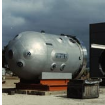
(E&TR November 1989) The Laboratory's High Explosives Applications Facility's (HEAF's) cylindrical steel containment vessel, 3.6 m in diameter and 12 m long, shown prior to installation. It is used in experiments with a 100-mm-bore gun and for detonations of up to 5 kg of high explosives (TNT equivalent), but will be upgraded to withstand detonations of up to 10 kg.
