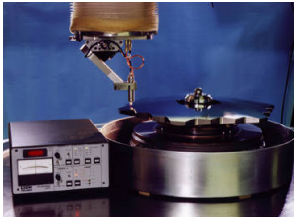
Figure 4. The amplifier (left), shown next to a part under inspection; the LVDT probe extends from the tool bar of the Large Optics Diamond Turning Machine. The part under inspection is the Keck II secondary mirror for the Keck Observatory in Hawaii.
