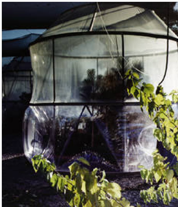
The elevated CO 2 exposure facility at LLNL is allowing us to study the differences between conifer seedlings growing under ambient conditions and those growing under elevated levels of CO 2 .
