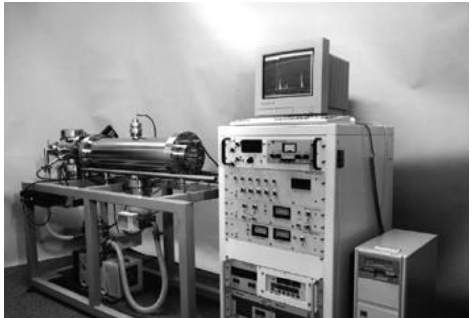
Figure 3. Our laboratory-size ion-storage trap/time-of-flight (IT/TOF) instrument. We are currently designing a smaller transportable instrument.
