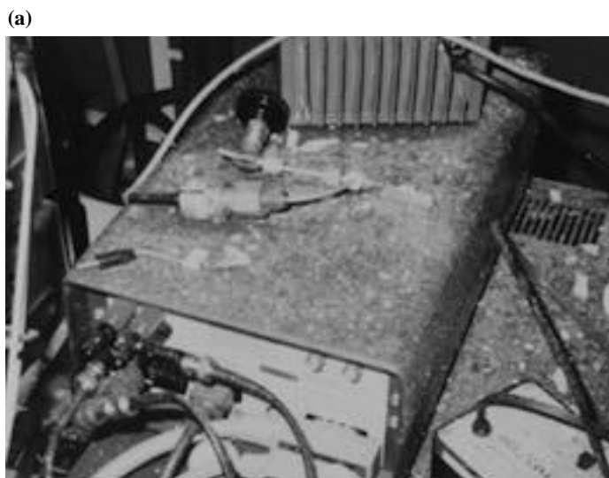
Figure 5. In 1992, an explosion occurred during a "cold-fusion" experiment at a research laboratory in California. About 65 LLNL scientists were called upon to analyze the debris (a) to shed light on potential causes of the explosion. The distended cold-fusion cell after the explosion is shown in (b). Our most unanticipated result was that machine-shop lubricating oil could have been a potential contributor to the incident. 1
