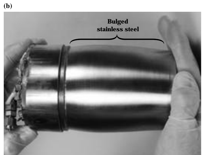
Figure 5. In 1992, an explosion occurred during a "cold-fusion" experiment at a research laboratory in California. About 65 LLNL scientists were called upon to analyze the debris (a) to shed light on potential causes of the explosion. The distended cold-fusion cell after the explosion is shown in (b). Our most unanticipated result was that machine-shop lubricating oil could have been a potential contributor to the incident. 1
