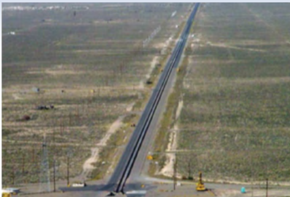
The sled test track at Holloman Air Force Base is 16 kilometers (10 miles) long.
