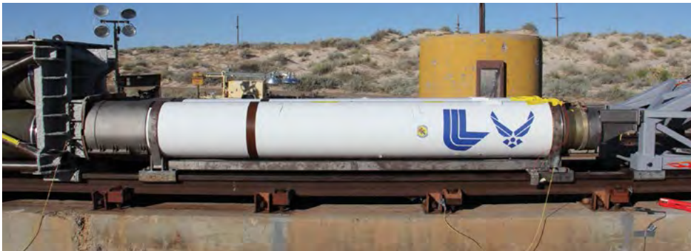
The forebody sled was propelled by two pusher stages. (top) In the first stage, four Nike rocket motors provided the initial thrust. (bottom) The second stage was loaded with two Super Terrier rocket motors.
