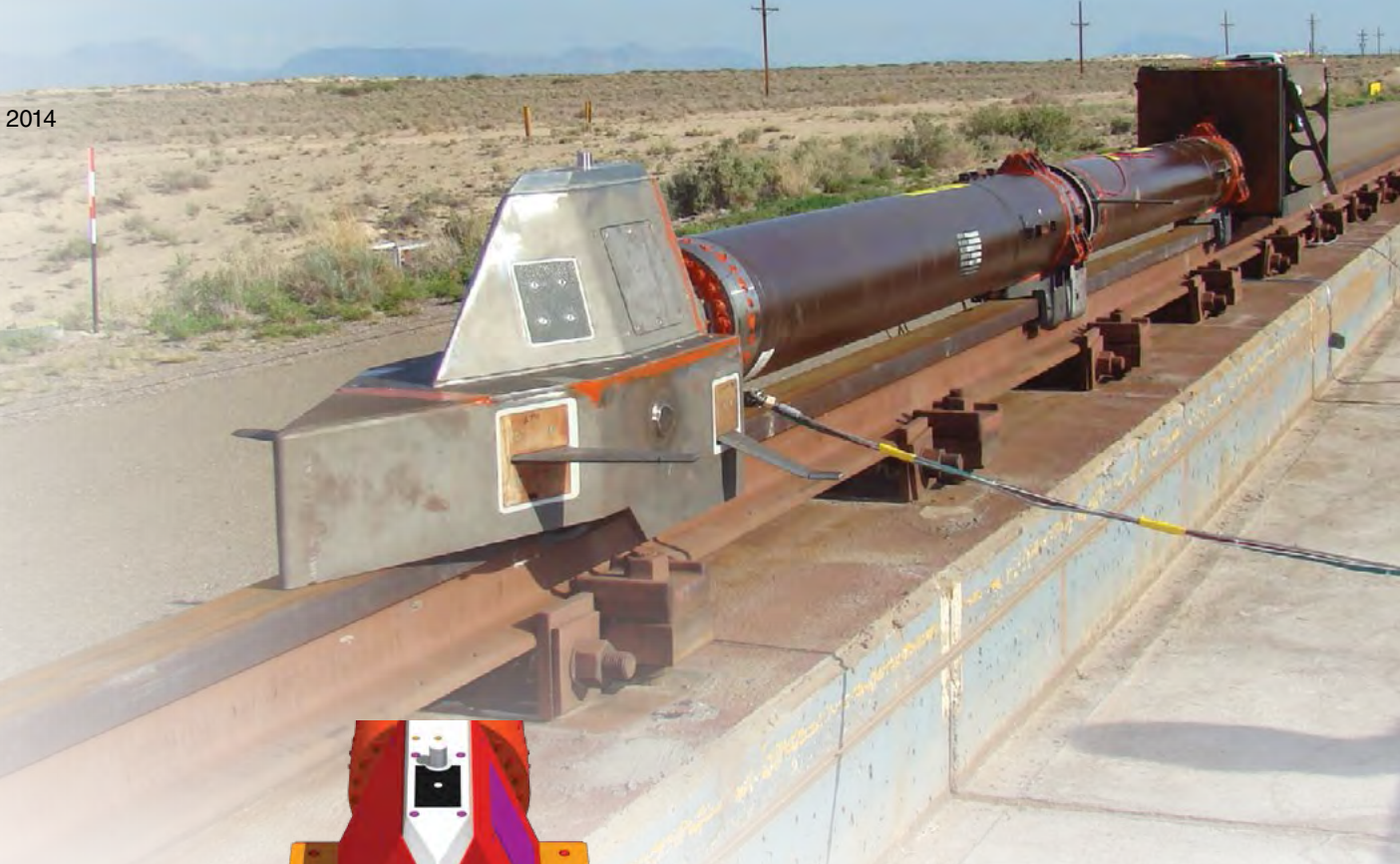
A monorail dry-run test at Holloman Air Force Base in July 2013 had no payload and used three representative carbon-epoxy panels mounted on the top and sides of the sled. (Rendering by Kwei-Yu Chu)
