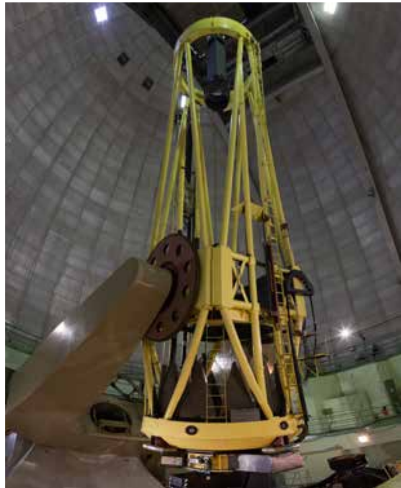
Lick Observatory’s 3-meter Shane telescope has been used for testing many new instruments for astronomy research, including the novel adaptive-optics-based laser guide star—developed with help from Livermore scientists. (Photo by Lanie L. Rivera.)
