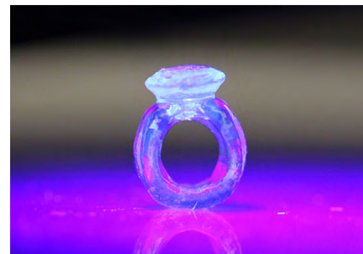
Livermore researchers can quickly 3D print stronger, more flexible objects from thiol-ene resins using CAL, a volumetric additive manufacturing (VAM) technology. (Photo by Maxim Shusteff.)
