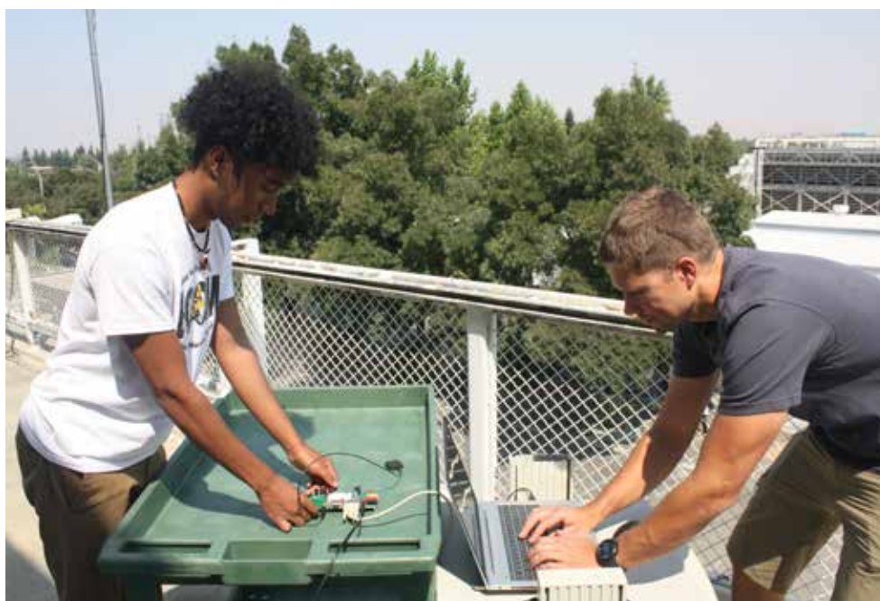
During a telemetry verification test of MiniCarb's satellite radio, physicist and engineer Lance Simms (right) and engineering summer student Nicholas Hsiao send a communication signal to the Iridium satellite network in space. The signal is relayed back to them via a ground station. (Photo by Dan Linehan.)
