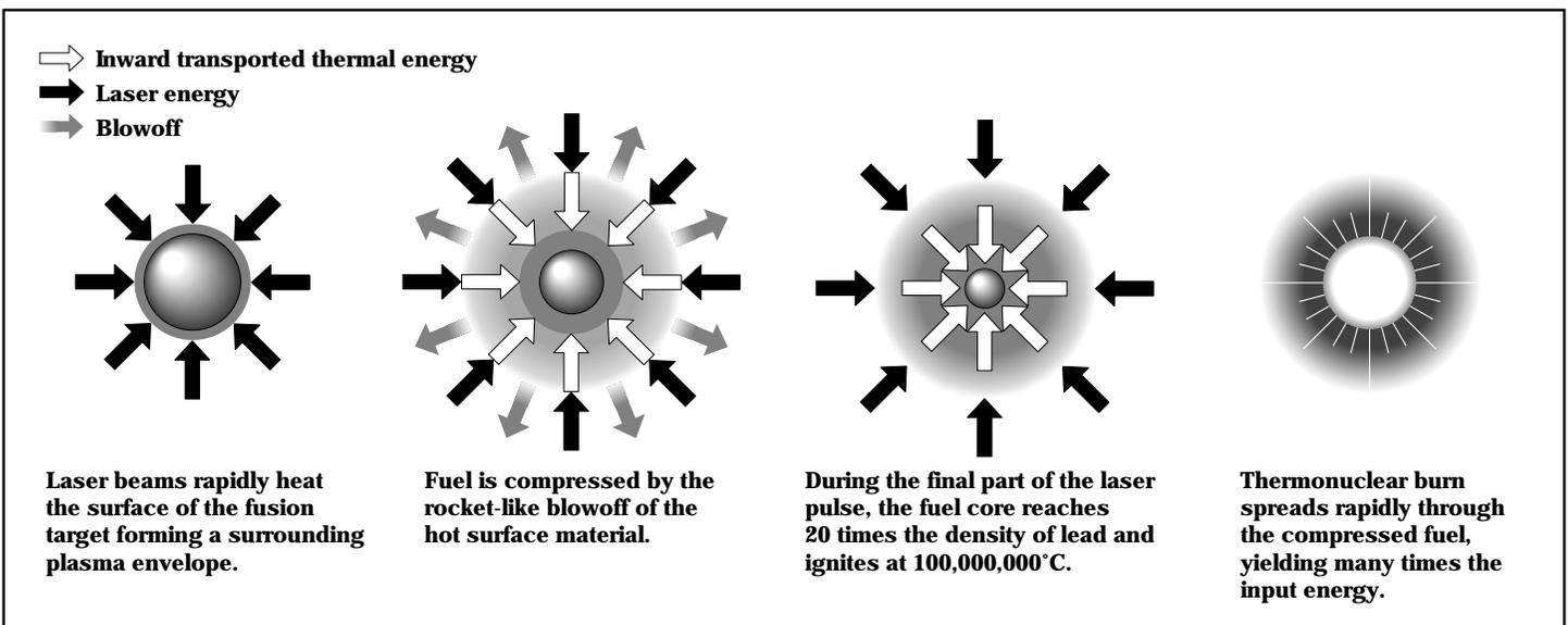
**Figure 4.** The steps of an inertial confinement fusion reaction, which produces up to ten times the energy used to initiate ignition. Under laboratory conditions, the sequence produces energy gain equivalent to the power of a miniature star lasting for less than a billionth of a second.
