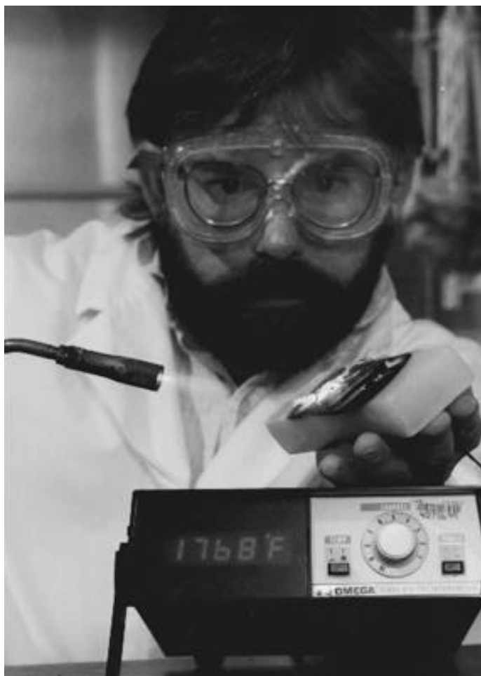
Figure 6. Tom Tillotson, a chemist at LLNL, applies a propane torch to the top of a 2.5-cm-thick silica aerogel brick. His hand remains totally unaffected by the heat.
