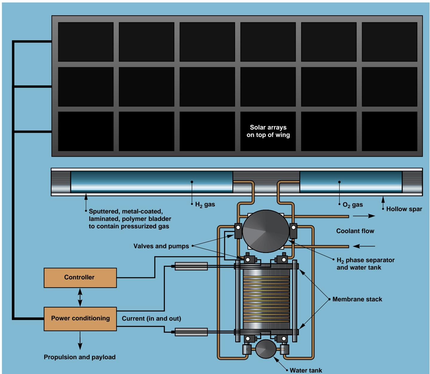
Figure 6. Rendering of a generic unitized regenerative fuel cell subsystem, including storage of reactant gases in the wing spar.
