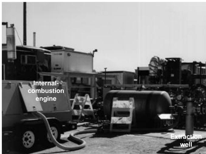
**Figure 4.** View of the vapor-extraction treatment system. The internal combustion engines inside the trailer create the underground vacuum; the engines run directly off gasoline vapors pulled from the extraction wells.
