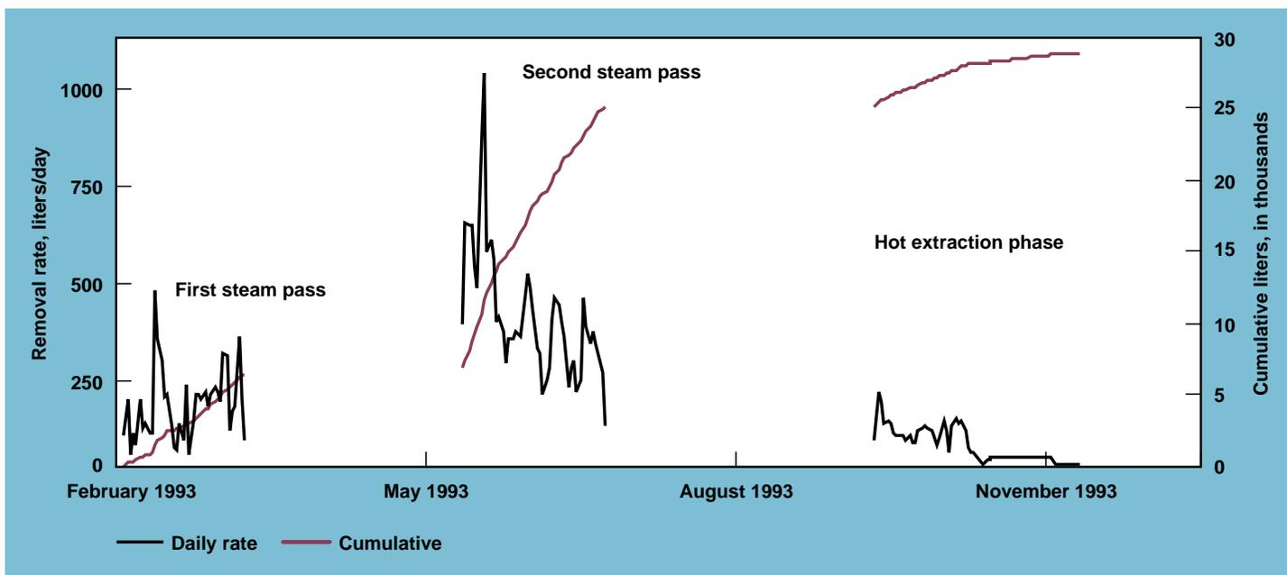
**Figure 3.** Daily extraction rates and cumulative volumes of extracted free-product gasoline show the three extraction phases. Extraction rates were highest during the second phase, when extraction systems were optimized and we used a pulsed mode of operation, alternating steam injection and vacuum-only phases.
