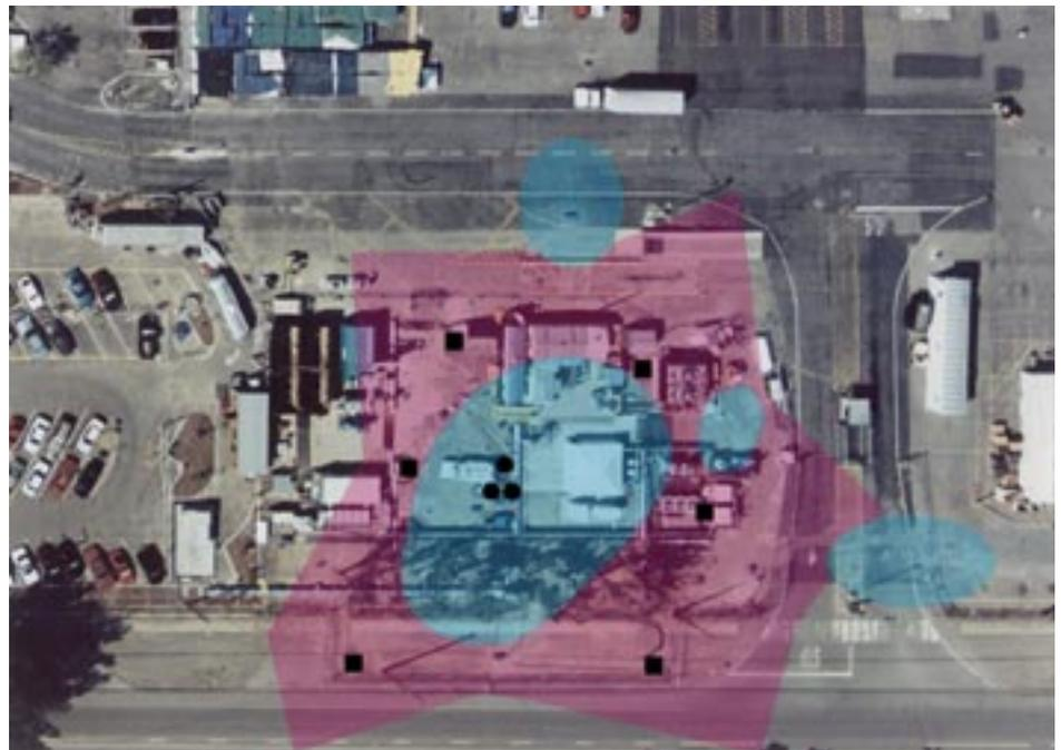
**Figure 2.** Top view of LLNL spill area, showing regions of known or suspected free-product gasoline contamination (circled in blue) and where we applied dynamic underground stripping (in pink). As noted by the circles outside the treatment area, additional free-product gasoline remains at the site.
