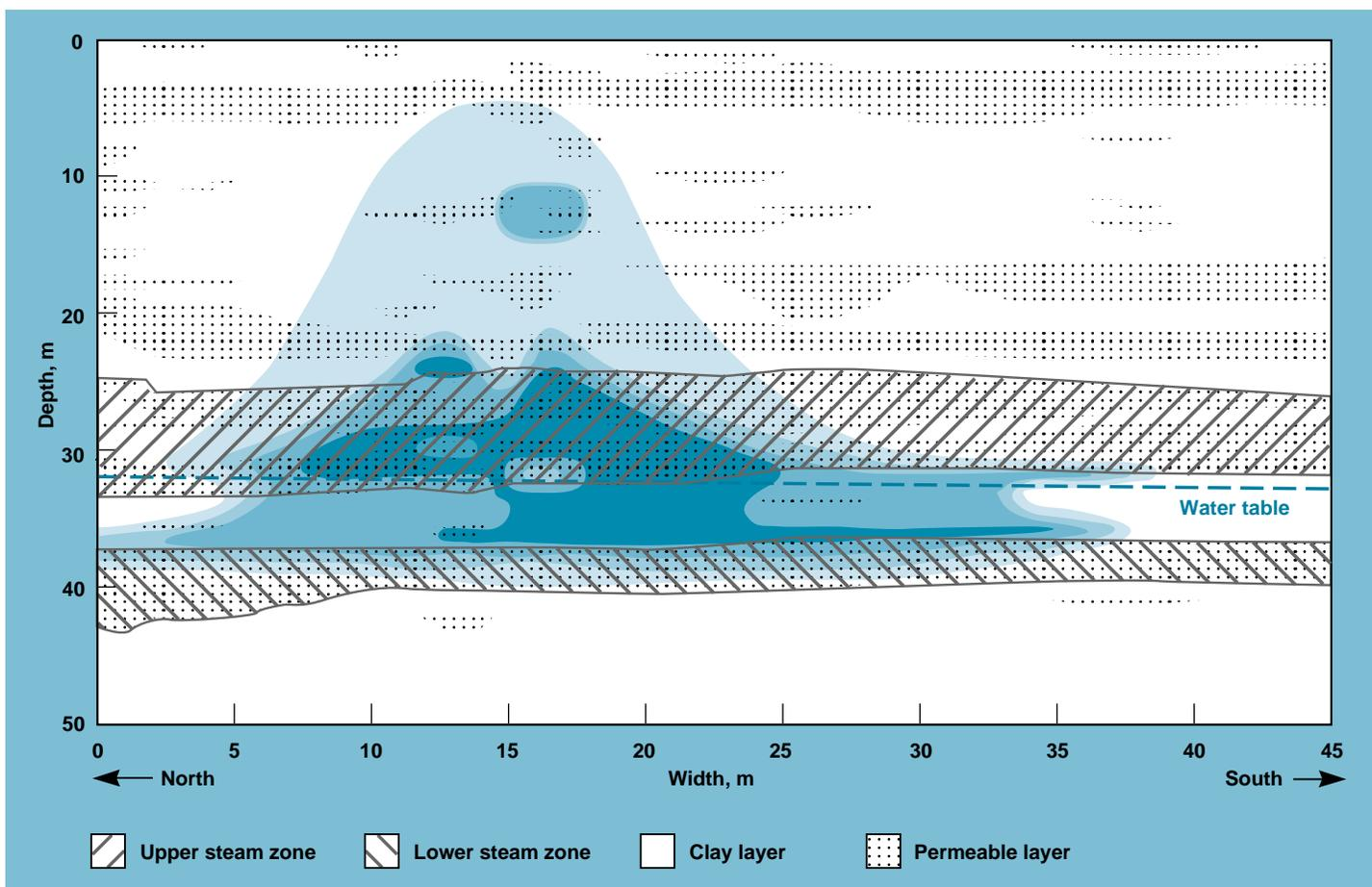
**Figure 1.** Cross section showing an approximation of the gasoline contamination at the treatment site before dynamic underground stripping began. The darker areas represent higher concentrations or free-product gasoline. The dashed line denotes the level of the water table.
