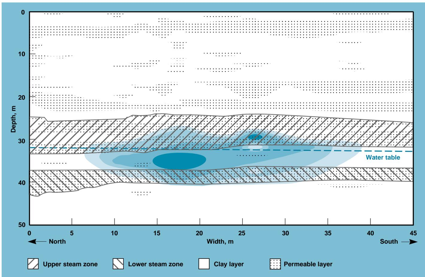
**Figure 5.** Approximate cross section of the treatment site after the two steam passes (compare with Figure 1). The area of gasoline contamination has contracted greatly.
