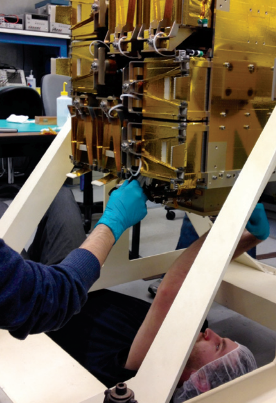
The STARE CubeSats are integrated into the main box that bolts to the launch vehicle.
