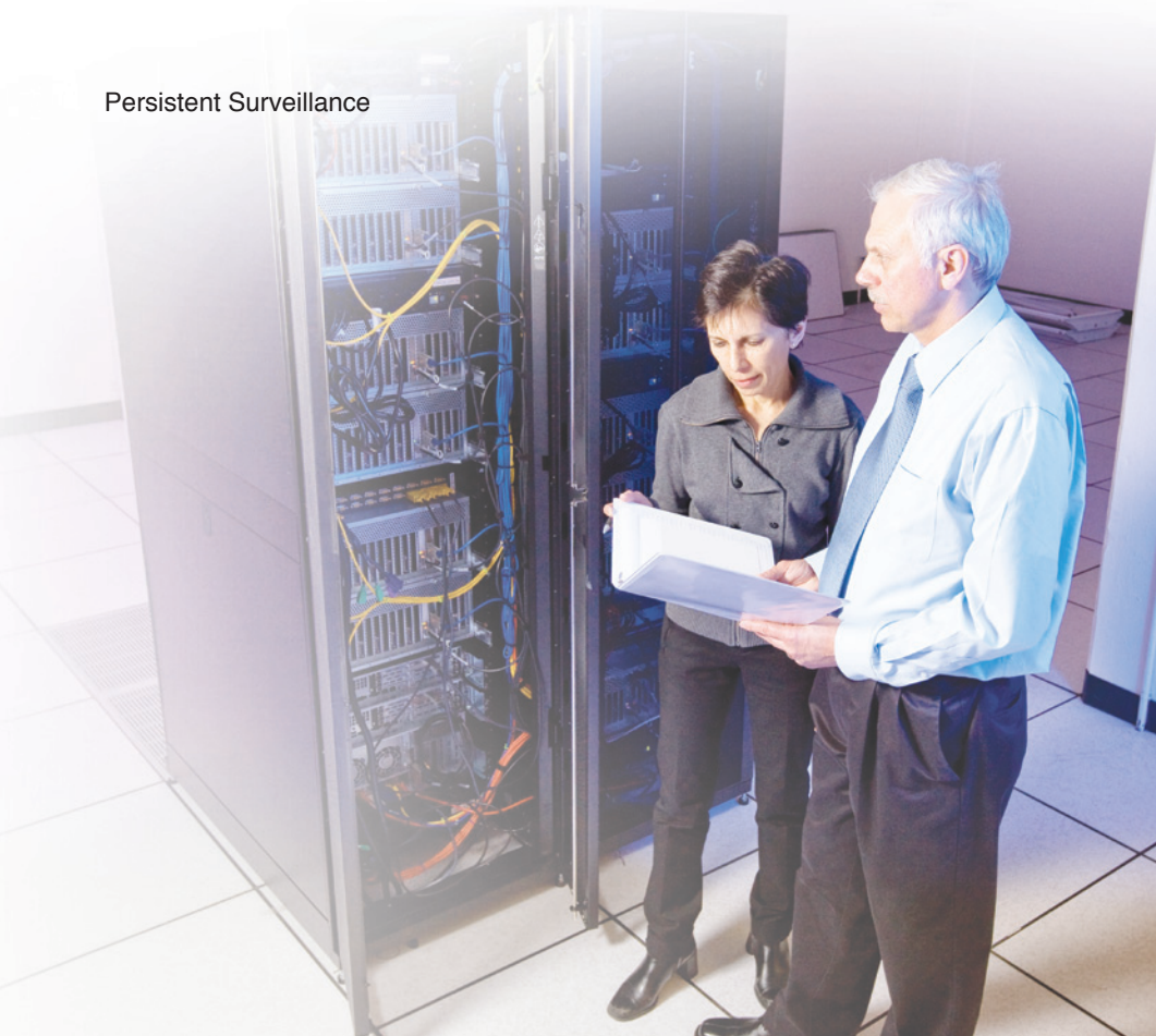
Persistics software is currently housed on a high-density 12-node miniclust, providing an aggregate 40 trillion floating-point operations per second of computing capability. Each node contains a combination of central processing units and seven graphics processing units. Pictured are (left) Sheila Vaidya and Holger Jones.
