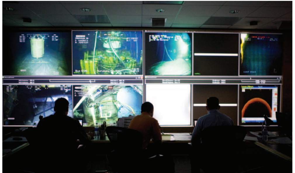
BP’s crisis command center in Houston, Texas, was called the HIVE because it offered a highly immersive visualization environment. From these consoles, command center staff controlled 40 to 60 ships and 12 to 16 ROVs during containment and oil-recovery operations. (Courtesy of BP PLC.)
