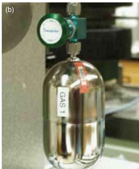
(a) The solid-phase microextraction (SPME) technique uses a tiny metal fiber coated with a polymer to adsorb organic compounds liberated in a weapon’s headspace. The retrieved needle is inserted into a gas chromatograph–mass spectrometer to obtain a chemical analysis of the weapon’s internal environment. (b) For more extensive analysis, chemist Chris Harvey developed a method to conduct SPME “offline” using a 400-milliliter container to hold the gas taken from a warhead. In a laboratory setting, several samples can be extracted for repeated analyses to build a database of compounds.
