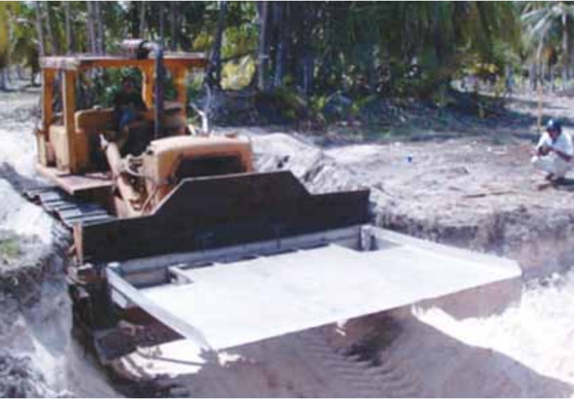
On Bikini Island, a large-plate lysimeter collects water from soils to determine the concentration of radionuclide contaminants present in that water. Lysimeter studies are providing data on the rainfall removal rate of cesium-137 from surface soils.
