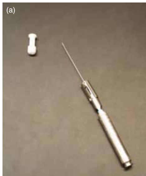
(a) The solid-phase microextraction (SPME) technique uses a tiny metal fiber coated with a polymer to adsorb organic compounds liberated in a weapon’s headspace. The retrieved needle is inserted into a gas chromatograph–mass spectrometer to obtain a chemical analysis of the weapon’s internal environment. (b) For more extensive analysis, chemist Chris Harvey developed a method to conduct SPME “offline” using a 400-milliliter container to hold the gas taken from a warhead. In a laboratory setting, several samples can be extracted for repeated analyses to build a database of compounds.
