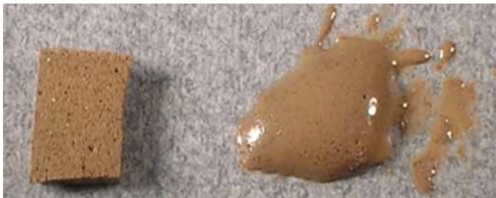
Polymer compatibility is critical to a weapon’s overall state of health. This example shows a sample of the polymer syntactic polysulfide, before (left) and after (right) exposure to an incompatible polymer.
