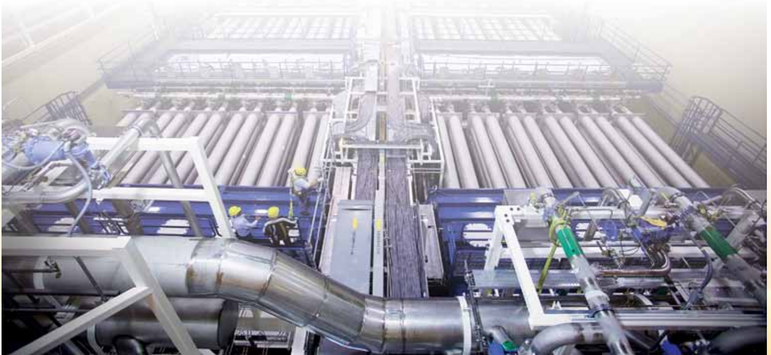
(above) The building housing the 192-beam laser and its target chamber is the size of three football fields. (below) Each of NIF's two identical laser bays has two clusters of 48 beamlines, one on either side of the utility spine running down the middle of the bay.
