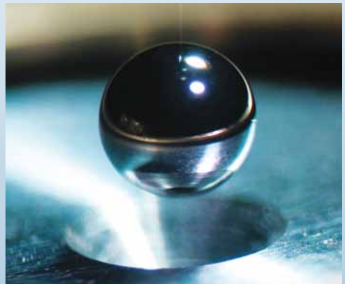
This polished capsule designed for inertial confinement fusion experiments is just 2 millimeters in diameter.
