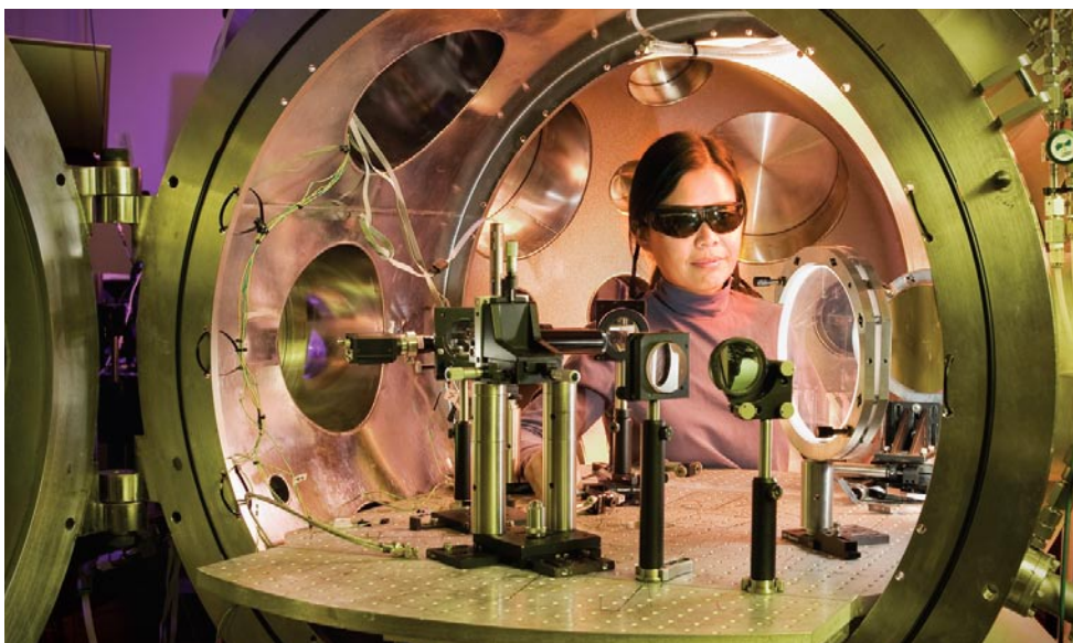
Physicist Hui Chen adjusts the optics in the target chamber of Livermore's Callisto laser during a proton acceleration experiment using a reduced-mass target.
