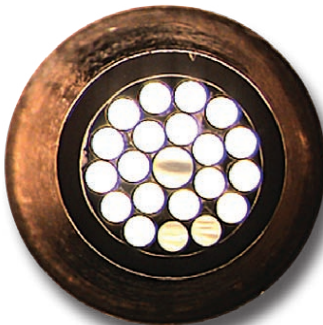
This prototype of a Livermore-designed sensor uses 20 glass fibers, each 300 micrometers in diameter, surrounding a fiber in which laser light illuminates gas contained in a glass capillary. The center fiber is 420 micrometers in diameter.
