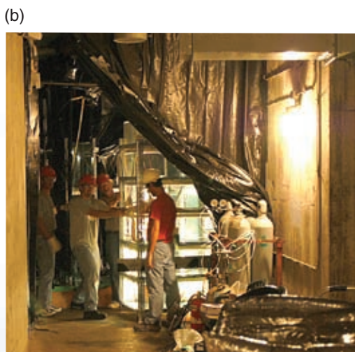
(a) For the field tests, detector prototypes are housed in the tendon gallery at SONGS. (b) The tendon gallery is a ring-shaped area about 10 meters underground and 25 meters from the reactor core.
