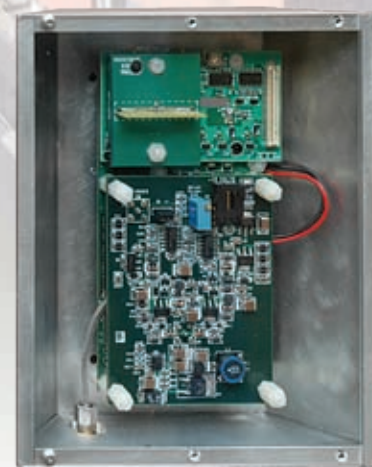
SecureBox is a wireless device that can be installed on cargo containers to detect intrusions.
