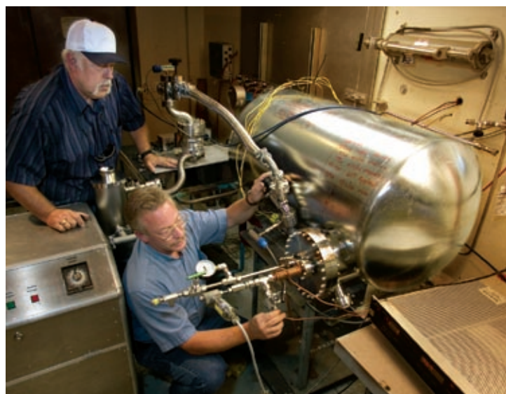
Vern Switzer (left) and Tim Ross check the pressure on the inner vessel that holds hydrogen of any temperature.
