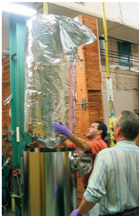
Francisco Espinosa-Loza (left) and Tim Ross lower the inner pressure vessel, insulated with reflective sheets of aluminum and plastic, into the outer stainless-steel vacuum jacket.
