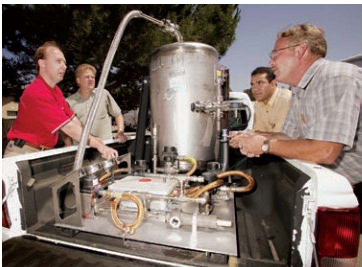
Left to right: Mark McCuller, Jim Fugina, Francisco Espinosa-Loza, and Tim Ross worked on the first-generation design of the Livermore hydrogen storage system, which was installed in the back of a Ford Ranger pickup.
