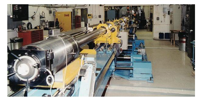
The two-stage gas gun at the Joint Actinide Shock Physics Experimental Research Facility in Nevada is one method used to perform shock physics experiments. (Photograph courtesy of the Nevada Test Site.) Each month in this space, we report on the patents issued to and/or the awards received by Laboratory employees. Our goal is to showcase the distinguished scientific and technical achievements of our employees as well as to indicate the scale and scope of the work done at the Laboratory.
