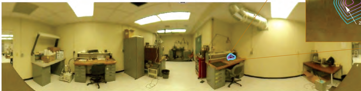
A Compton imager combined with a camera produced this image, which pinpoints the location of the radioactive source—an isotope of sodium ( ^{22}\text{Na} ).
