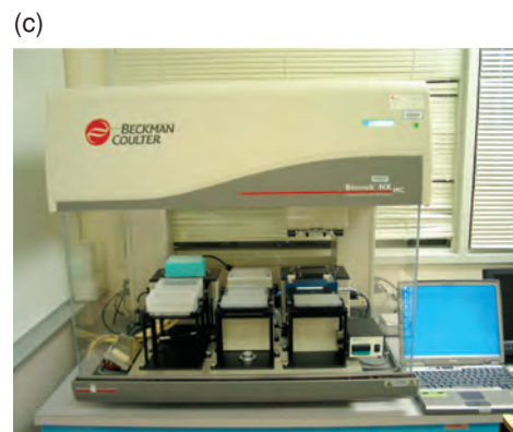
(a) A specialized flow cytometer, the Bio-Rad Bio-Plex Workstation, analyzes DNA using bead-based liquid array technology by Luminex Corporation. (b, c) To speed diagnosis during a disease outbreak, Livermore researchers designed robotic equipment to replace most manual operations.
