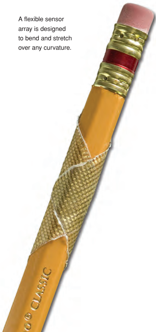
Serpentine gold wires, each encased in polyimide, connect "islands" of silicon stress sensors.
