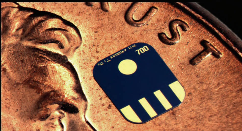
One stress sensor measures just 4 millimeters square and 50 micrometers thick.
