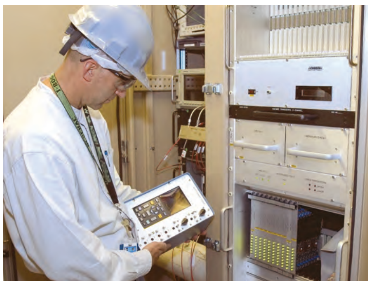
Livermore engineer Rob Hartley tests a beam-control front-end processor, which is used to position motors in the alignment system.
