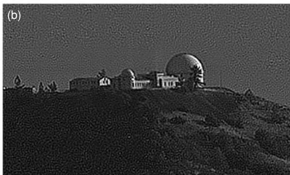
Livermore researchers imaged the University of California's Lick Observatory on Mount Hamilton with a remote-surveillance system from 60 kilometers away. (a) The unprocessed image is blurry. (b) The image produced using the speckle-processing technique is much clearer.
