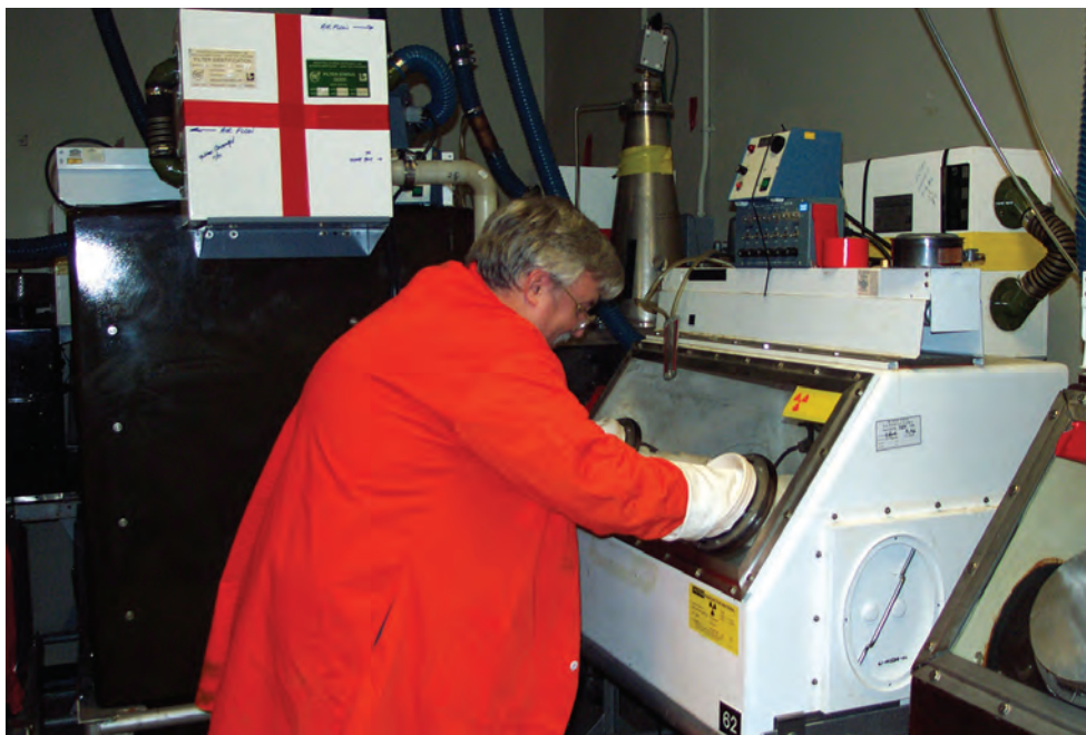
Livermore nuclear chemist Ken Moody performs forensic radiochemical analysis on samples inside a glovebox. The procedures for working with radioactive samples ensure a safe working environment and maintain the integrity of the samples.
