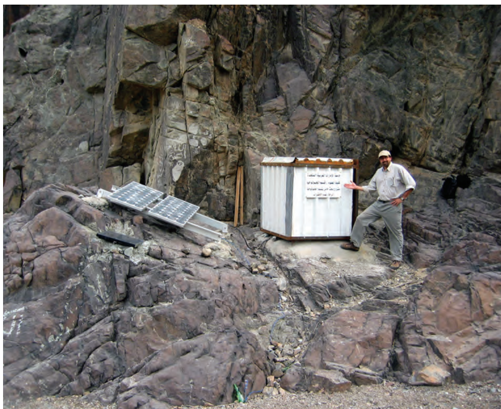
Livermore seismologist Arthur Rodgers checks on a seismic station erected at Al Hayl, United Arab Emirates, as part of a joint project between the Laboratory and United Arab Emirates University. The enclosure contains seismic equipment powered by the solar cell to the left.
