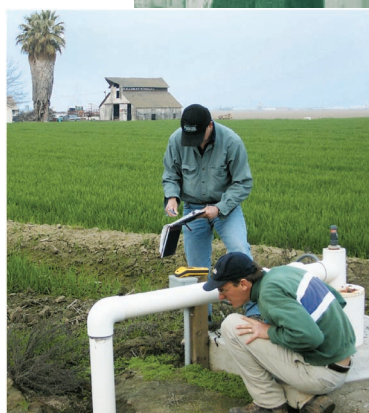
Livermore researchers are installing a network of multilevel monitoring wells near a dairy farm in California’s Central Valley so they can study the groundwater flow paths, nitrate transport, and denitrification. The arrow shows the direction of groundwater from an irrigation canal toward the monitoring wells. Manure used on crops is one possible source of nitrate found in groundwater.
