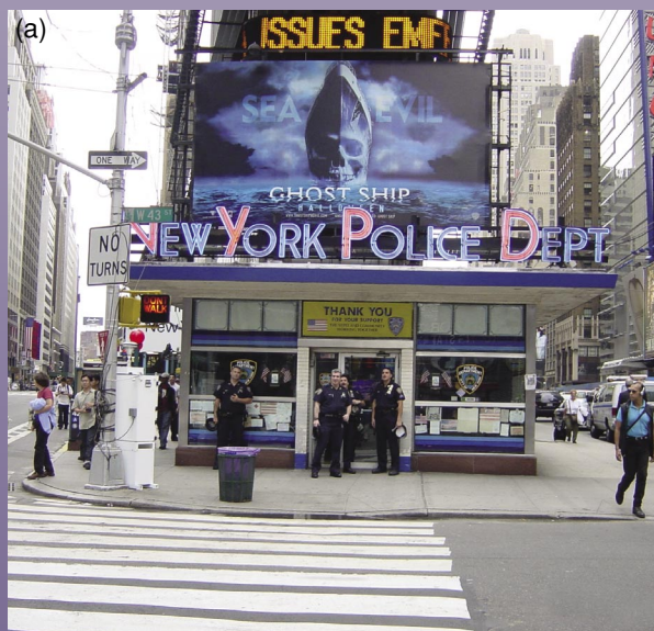
(a) Air samples are collected by this BASIS sensor installed outside a New York Police station. (b) Another sensor resides in a New York City borough neighborhood. (c) New York City Department of Public Health officers accompany a Department of Energy employee retrieving air samples from a sensor located near the former World Trade Center. Air samples are tested by Livermore technicians at a nearby laboratory.
