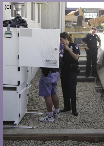
(a) Air samples are collected by this BASIS sensor installed outside a New York Police station. (b) Another sensor resides in a New York City borough neighborhood. (c) New York City Department of Public Health officers accompany a Department of Energy employee retrieving air samples from a sensor located near the former World Trade Center. Air samples are tested by Livermore technicians at a nearby laboratory.
