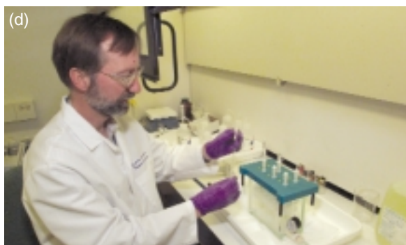
(a) Chemist Armando Alcaraz logs in a proficiency test sample. (b) Chemist Bob Maxwell holds a sample in a tube that will be placed in a nuclear magnetic resonance instrument (in background). (c) Alcaraz injects a microliter of sample into a gas chromatograph–infrared spectrometer system. (d) Chemist Hugh Gregg uses solid-phase extraction cartridges to clean a sample of hydrocarbon compounds that might mask a chemical warfare agent.
