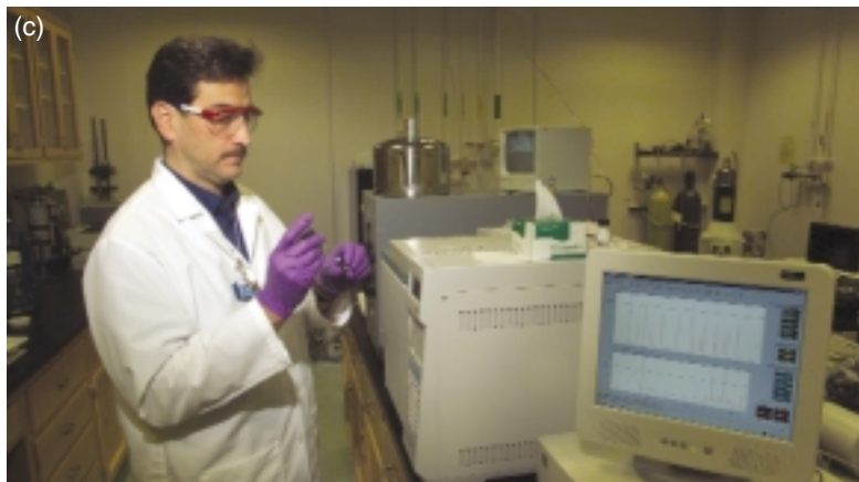
(a) Chemist Armando Alcaraz logs in a proficiency test sample. (b) Chemist Bob Maxwell holds a sample in a tube that will be placed in a nuclear magnetic resonance instrument (in background). (c) Alcaraz injects a microliter of sample into a gas chromatograph–infrared spectrometer system. (d) Chemist Hugh Gregg uses solid-phase extraction cartridges to clean a sample of hydrocarbon compounds that might mask a chemical warfare agent.
