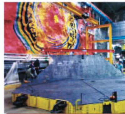
Two layers of steel plates (four plates per layer) are welded together on a detector frame.
