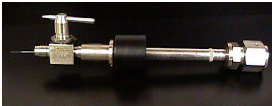
This solid-phase microextraction device is used to collect molecules that are formed or outgassed from the nuclear and thermal breakdown of organic polymers and high explosives contained in nuclear warheads. Signs of outgassing can indicate problems with parts that need to be replaced.
