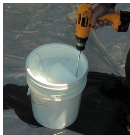
L-Gel is shipped premixed as a semisolid. It is relquefied to a house-paint consistency by vigorously shaking it by hand or using a power stirrer.
